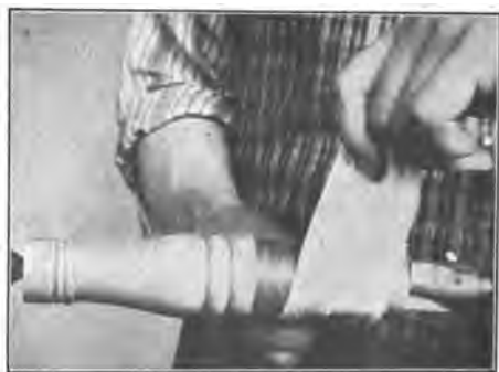
Fig. 71. Polishing with Cloth.
